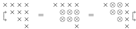
Figure 3: Transfer of a core transformation from the left of an upper triangular matrix to the right or vice versa.
